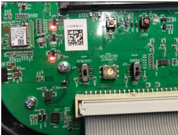
Close up RS485/ CAN bus switches
